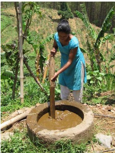
Stirring the dung and water before it's ready to supply methane gas to the kitchen
